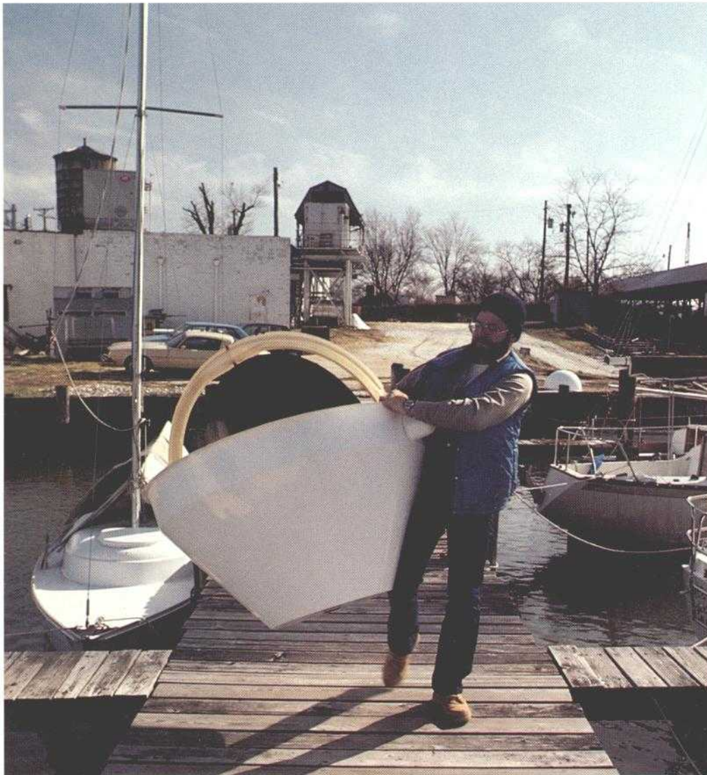
Facing Page. Above-decks assembly of new TeleSystems ship earth station taken apart to show graphite composite reflector. In the background, the Esperance. Left. TeleSystems' Ernest Peixotto shows just how lightweight above-decks assembly is.
