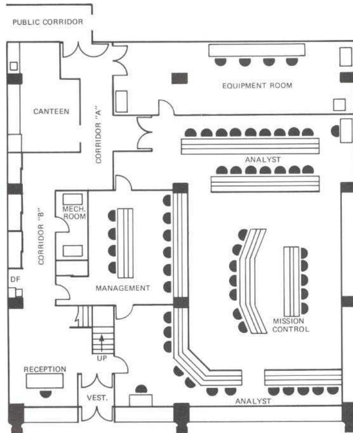
*Above: A diagram showing the layout of the first floor of the Launch Control Center. Photo left: The equipment room, which includes the center's two computers. Note TV cameras, top right.*
