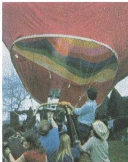
velope at the bottom and nearest the burners—is easily scorched. The crew must work quickly to keep the fabric away from the flame.
