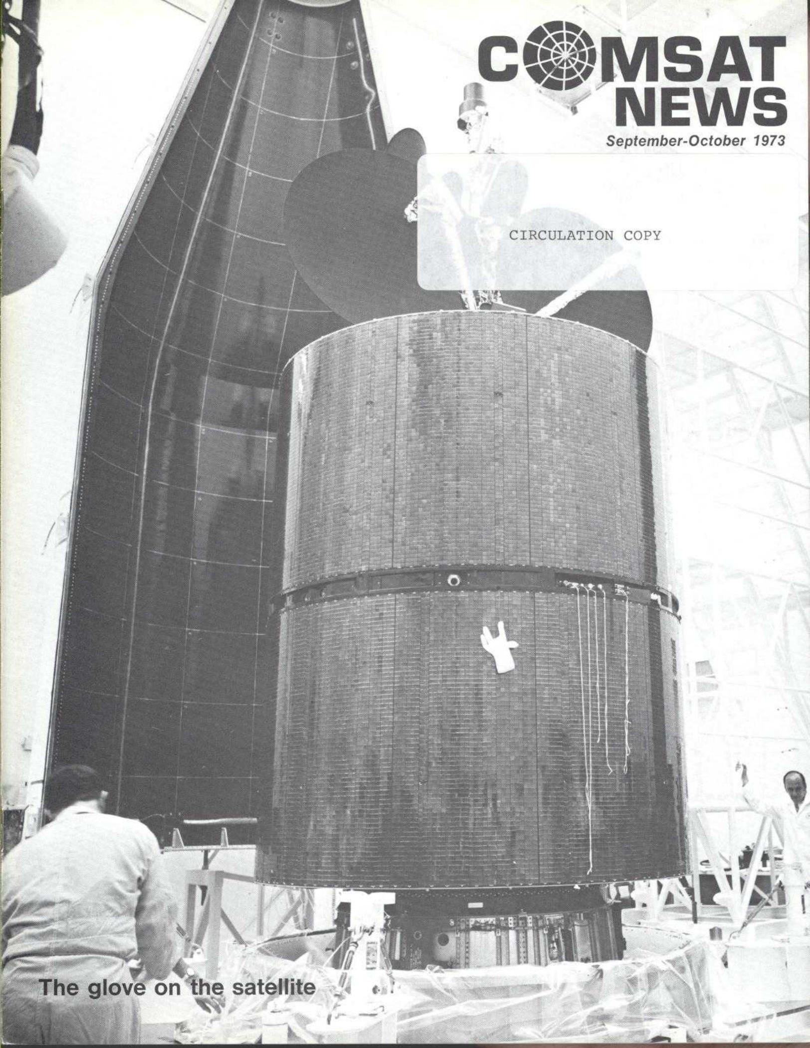
A large, dark, cylindrical satellite component is the central focus of the image. It is covered in a fine grid of solar cells. A white glove is placed on the surface of the component to provide a sense of scale. The component is being handled in a cleanroom environment, with workers in white protective suits visible in the background. The overall scene is brightly lit, highlighting the metallic and solar cell surfaces.
